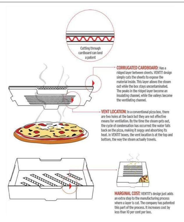
Figure 1: Ventit Design which helps to escape steam
